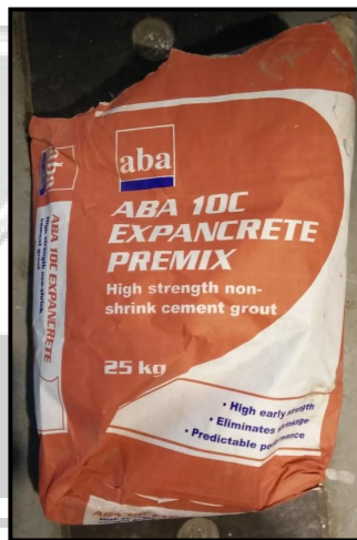
Figure 1: Non shrink grout used for infilling hollow core
