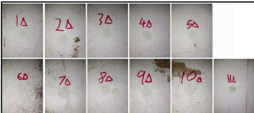
Figure 9: Perforation by small hard body impact - closed up view of indentations
