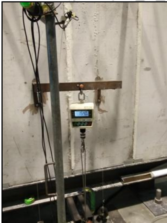
Figure 19: Heavy weight anchorage wash basin
