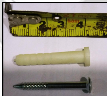
Figure 2: Screw with plastic anchor used for light weight anchorage tests
