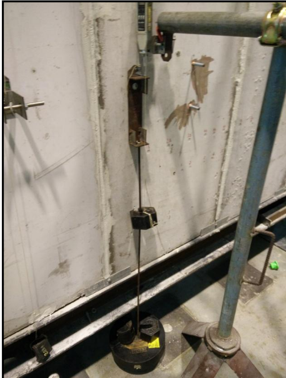
Figure17: Lightweight anchorage- pull-down test
