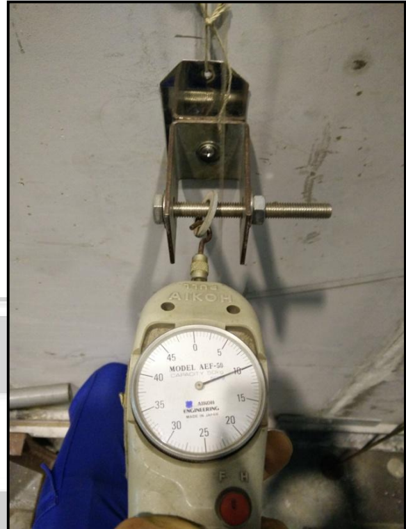
Figure 18 : Lightweight anchorage- pull-out test
